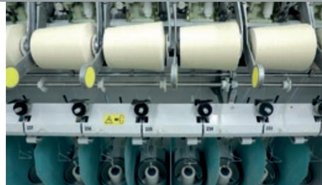
Savio's DUO POT system can be considered the real direct twisting of overlapped packages, it can be considered an “all-in-one” assembling and twisting.
