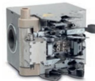
The consolidated experience on the splicer air technology in combination with the use of the heat, guarantees a final splice with excellent appearance, high and consistent strength even with difficult yarn structures, different blended materials and high twisted yarns.
