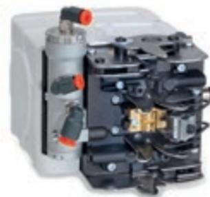
A common problem faced by the stretch fabric manufacturers is the breakage of the yarns during production. Savio offers a new splicing technology, combining air and water, which has given perfect results in this area.
